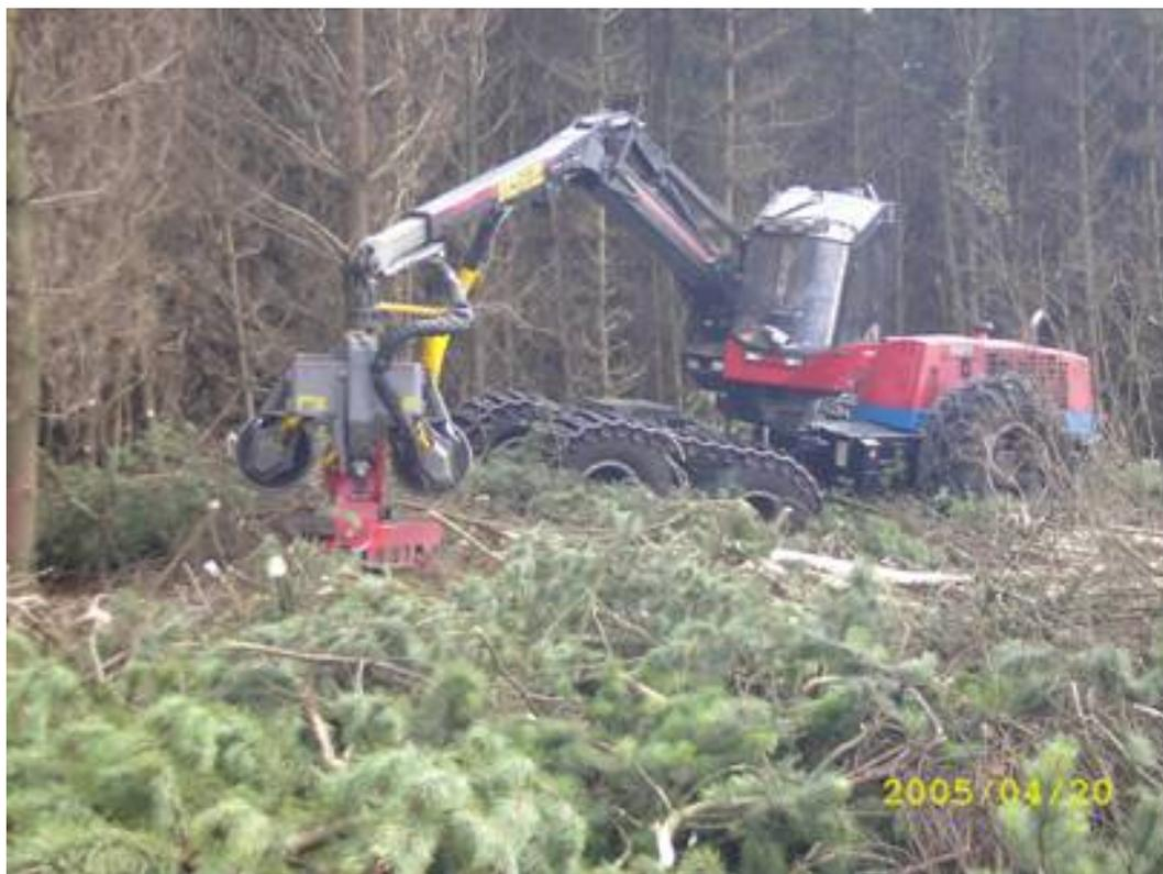
**Plate 15-1: Typical example of a Forest Harvester (Courtesy of Coillte)**
