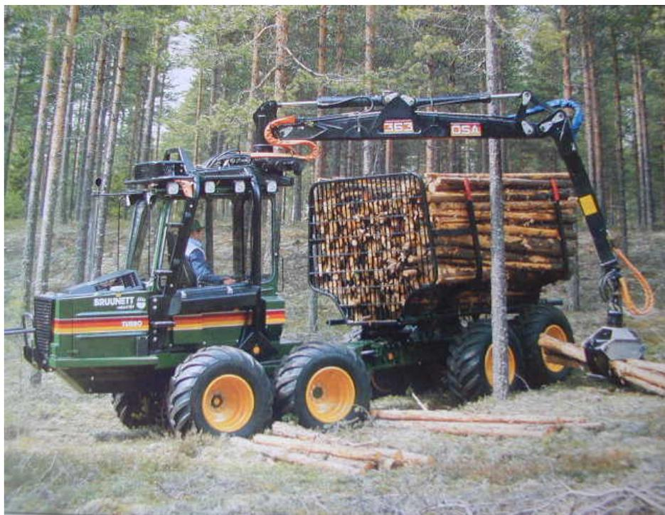
**Plate 15-2: Typical example of a forest forwarder (Courtesy of Coillte)**
